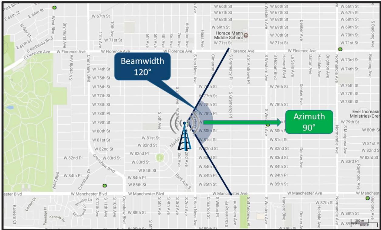
*Figure 3. Example of Azimuth and Beamwidth Measurements*
